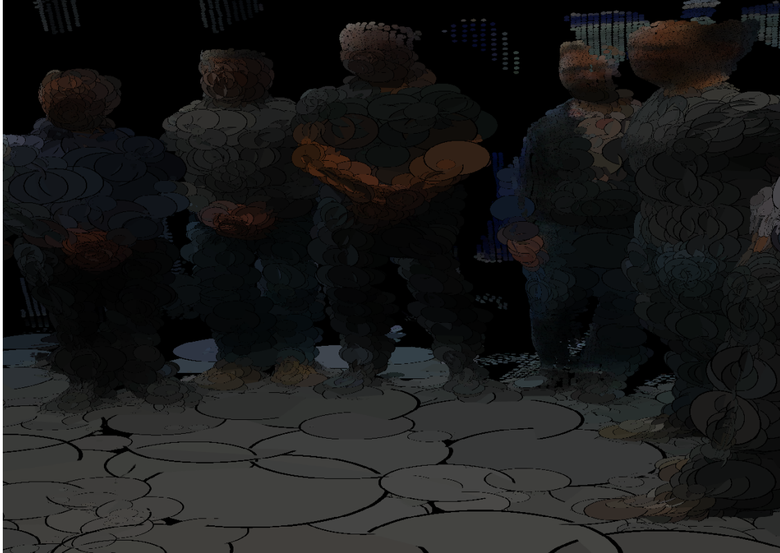
Figure 6.1: Simplified for3d_januartreffen point cloud. People are approximated by relatively small surfels, while the floor has larger uses fewer large surfels. Splats are outlined in black for better identification.
